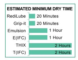
The chart below is designed to assist in determining the best P-80<sup>®</sup> for different applications. For most applications, the lubricants can be used interchangeably depending on the preference of the user.
